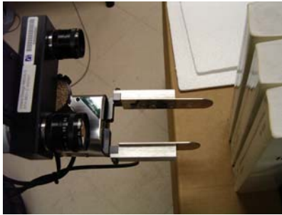
Figure 9. The “gripper” with the fingers specially designed.
