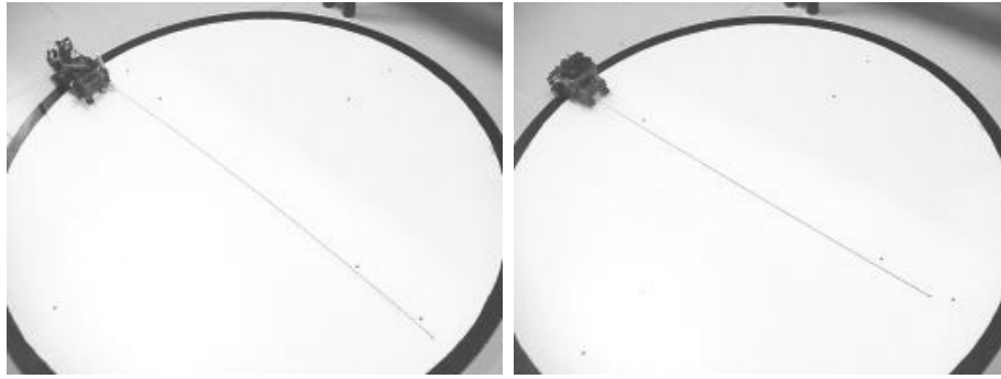
Figure 6. Trace of the robot for a commanded straight trajectory, using either a classic differential drive (left) or the new mechanical design (right).
